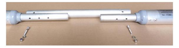
Longer antenna lower the resonance, shorter antenna increase the resonance. In both cases will have effect on the others lower bands. Start the eventual calibration always starting from the highest frequency (10m - 15m - 20m).
